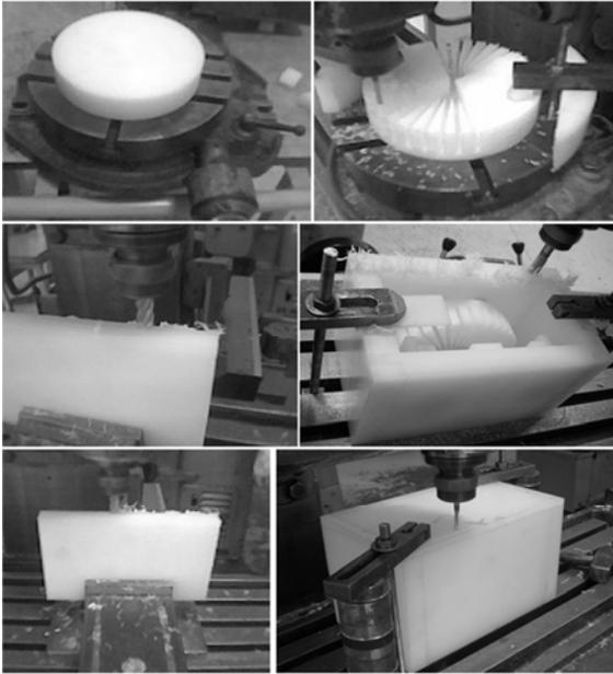
Figure 2. Milling of some phantom components.
