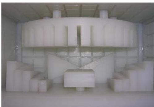
Figure 6. MTP phantom composed of - SL patterns, ST and N patterns, uniformity, S/N and  $f_0$  and other patterns.
